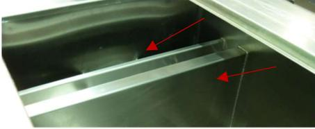
**IMPORTANT:** Always ensure both the main tank and auxiliary tanks are filled above the level marked. If not so, transducers and heating elements may get damaged.
