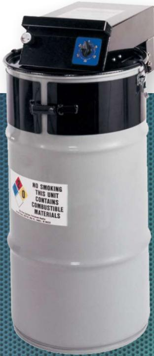
The Model 1670/1673 solvent parts cleaner is an immersion cleaner built for cleaning small parts typically found in automotive shops. The cleaner is designed to be placed on top of a 16 gallon drum and has a heavy duty motor for effective cleaning. Each model includes a rugged parts basket with 1/8" holes for smaller parts and a special hanger bracket.
