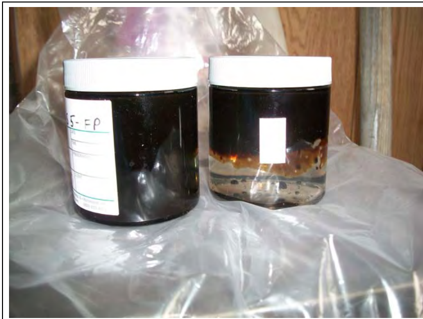
Photo 32: NAPL sample collected from T20S(5).
